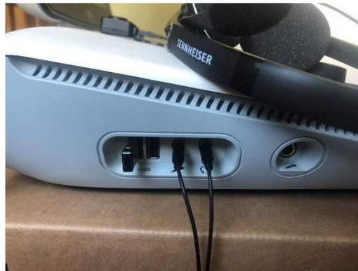
**Note:** The figure above shows the monitor cords and cables plugged into the side of the AudioStar audiometer (left side as viewed from the front).
