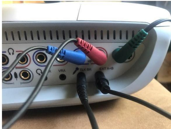
**Note:** The figure above shows a close-up view of all of these cords and cables plugged into the back panel of the AudioStar audiometer (right side as viewed from the back).
